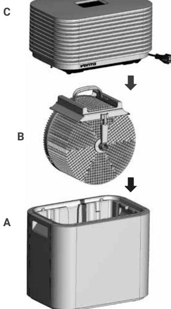
Place evaporation unit **B** into the water tray of the lower housing **A** and place upper housing **C** onto lower housing **A**, making sure it is the right way round.
